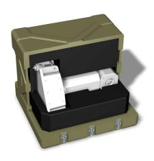
The elevation over azimuth Universal Sensor Platform Series USP-2x15 is driven by brushless servo motors, backlash free high reduction gear. Position is measured by direct mounted high resolution absolute encoder. The drive generates high torque, smooth rates and can tolerate load unbalances. Slip rings can be optional added for continuous rotation in the outer axis.
